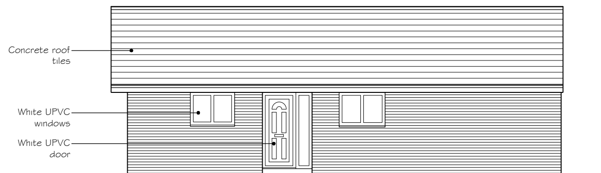
Existing Side (North West) Elevation (1:100)
