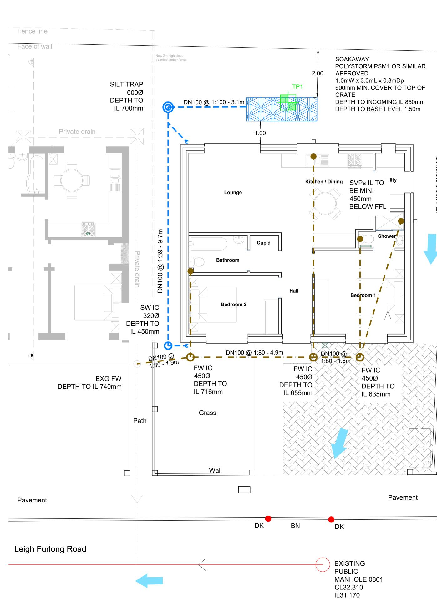
**INFILTRATION RATE 0.54m/hr** WAS USED BASED ON 3No. TEST RESULTS CARRIED OUT BY THE CLIENT.
