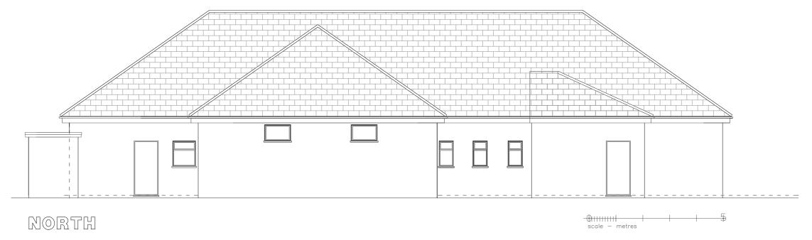
all doors and windows have existing security shutters as shown on south elevation
