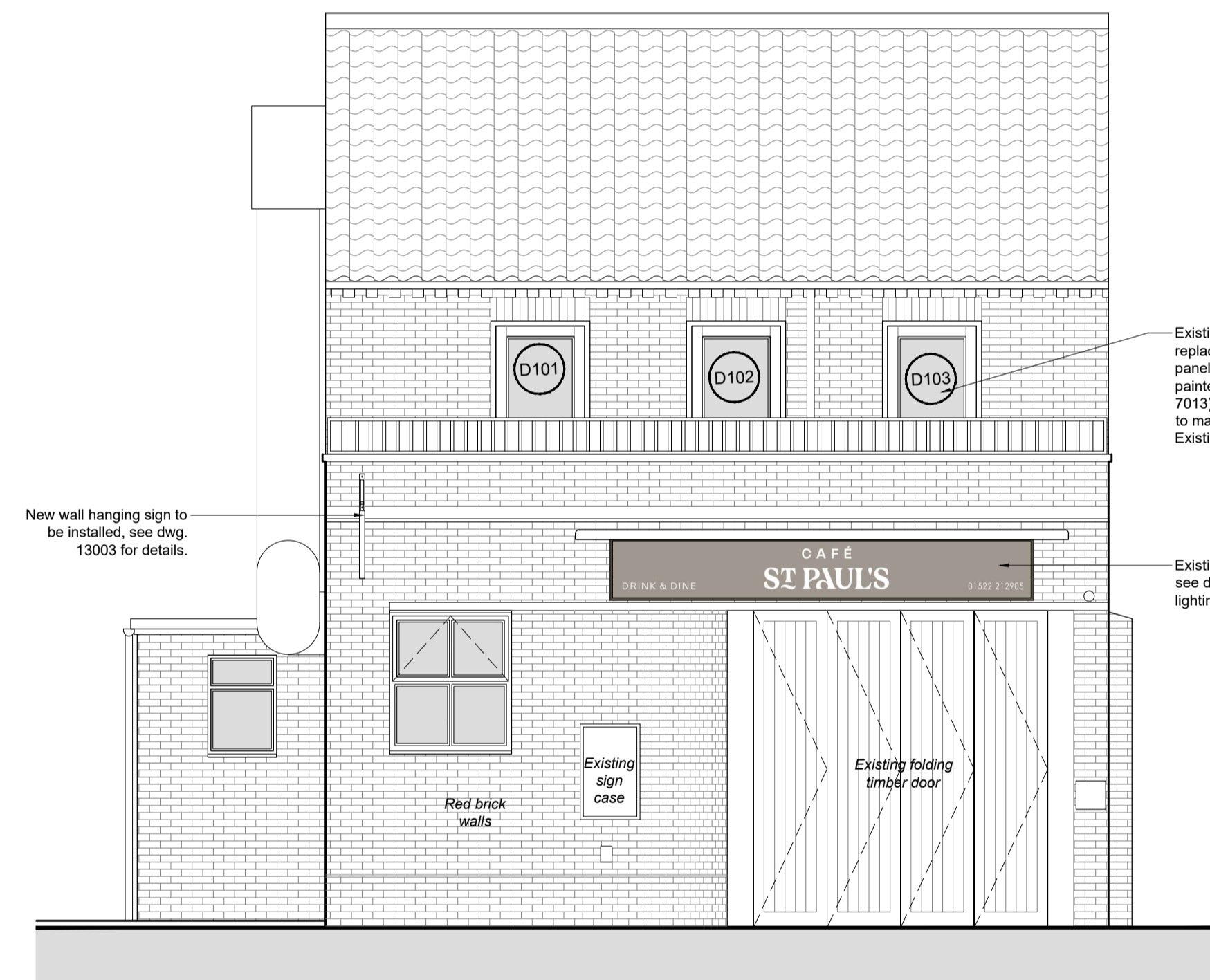
PROPOSED ELEVATION A (FRONT) 1:50 @ A1
