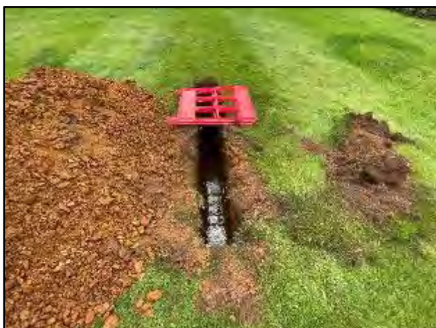
Photo 7 – A photo showing the material recovered from TP01 and the 'soakaway' infiltration testing.
