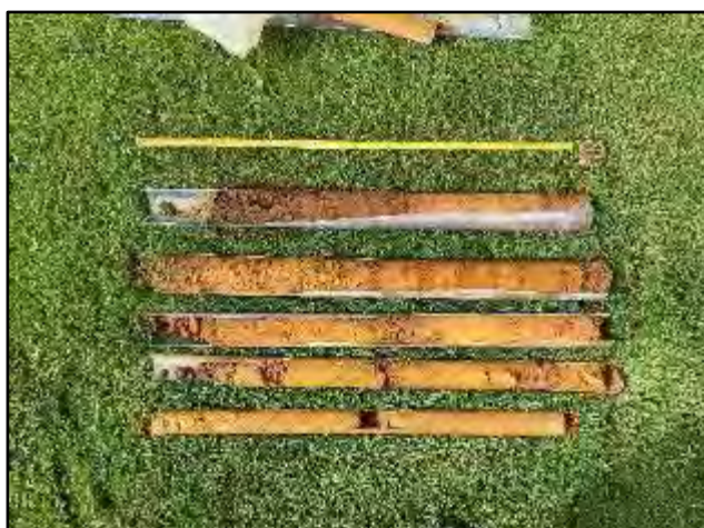
Photo 7 – A photo showing the material recovered from TP01 and the 'soakaway' infiltration testing.
