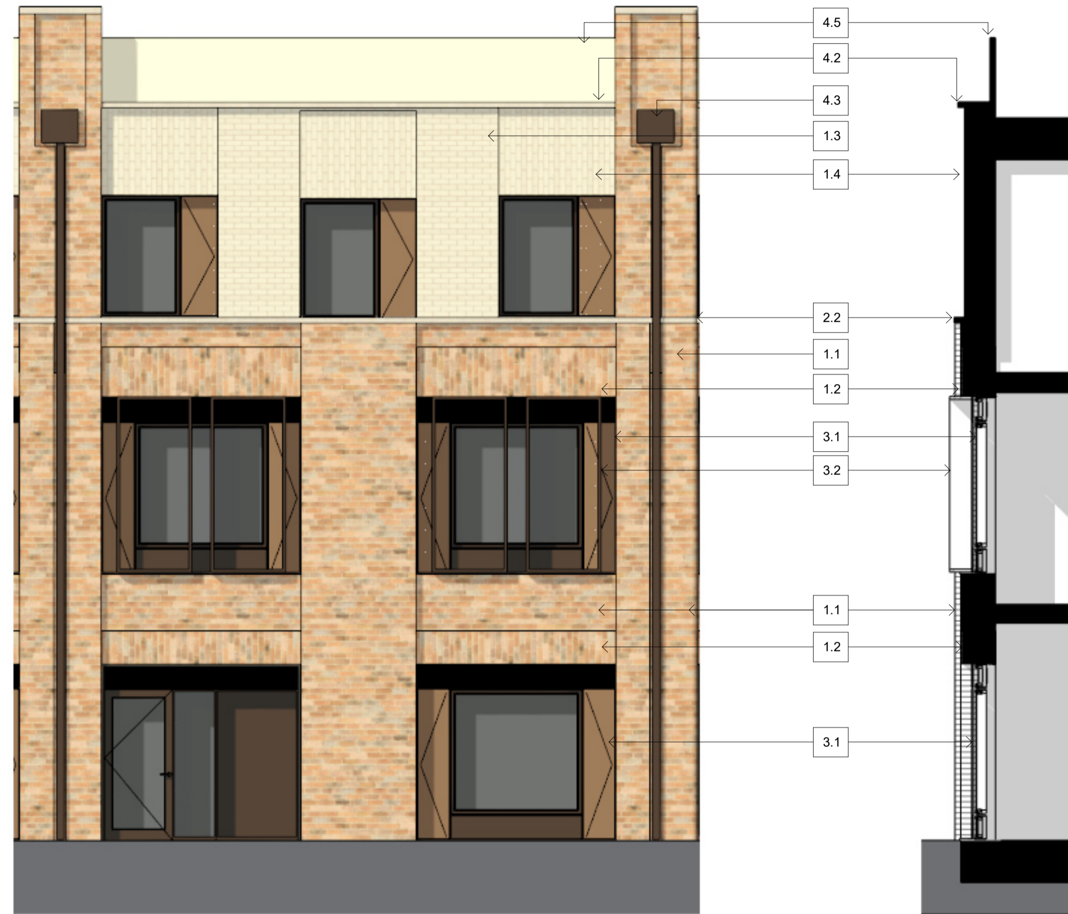
1 New Facade Elevation 2150 1 : 50
