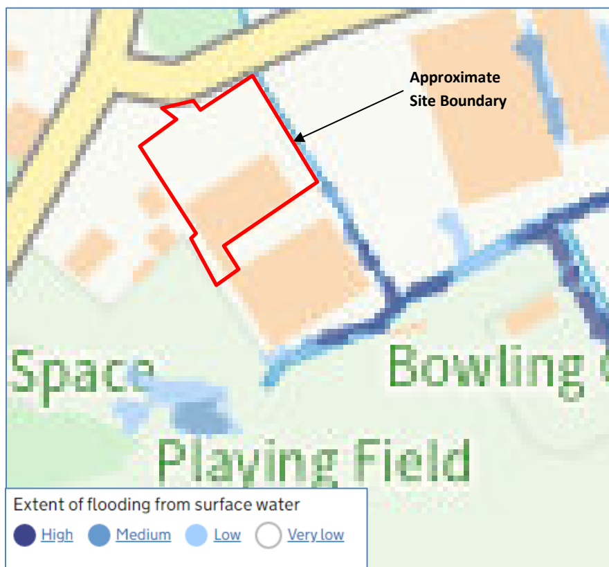
Figure 9.1 – Surface water flooding extents
