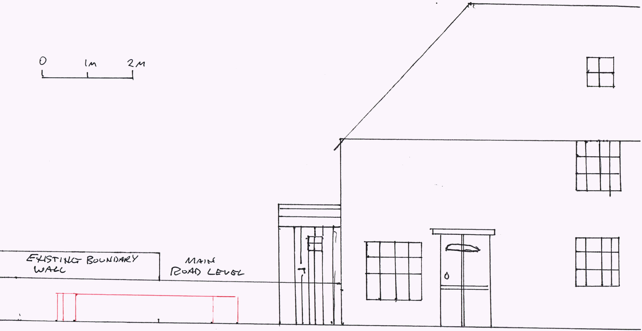
BROOKSIDE, MAIN ROAD SHAUFLEET, ISLE OF WIGHT, NORTH ELEVATION PROPOSED GARDEN BOUNDARY WALL SHOWN IN RED. SCALE 1:50
