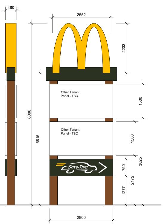
Steel frame clad in timber effect PCC aluminium with internally illuminated (static / 600cd/m2 (Max):
