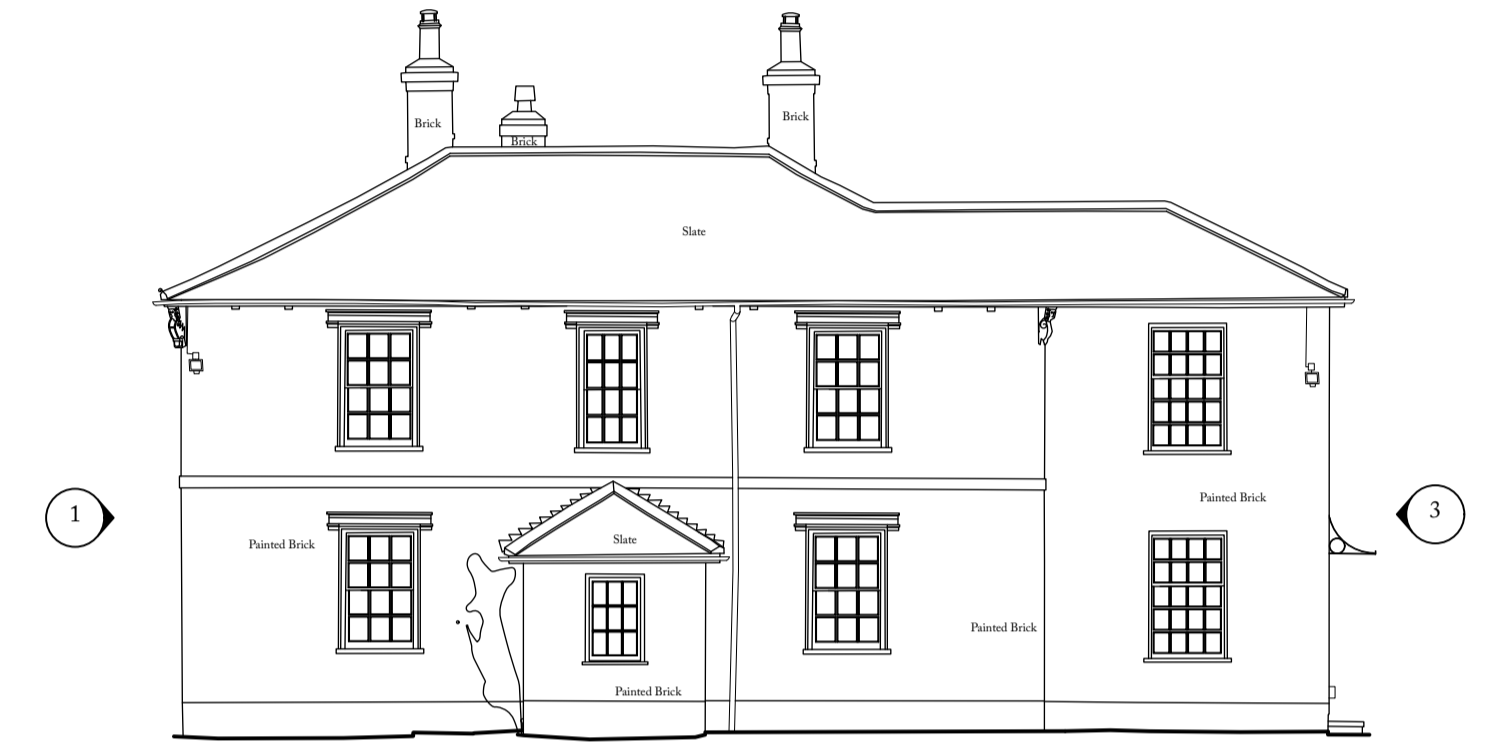
4 NORTHWEST ELEVATION As Existing, 1:100
