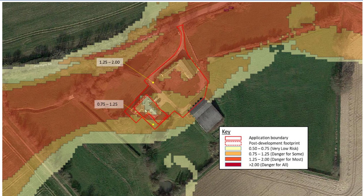
Figure 15 - Detailed surface water mapping – Low Risk Hazard Rating
