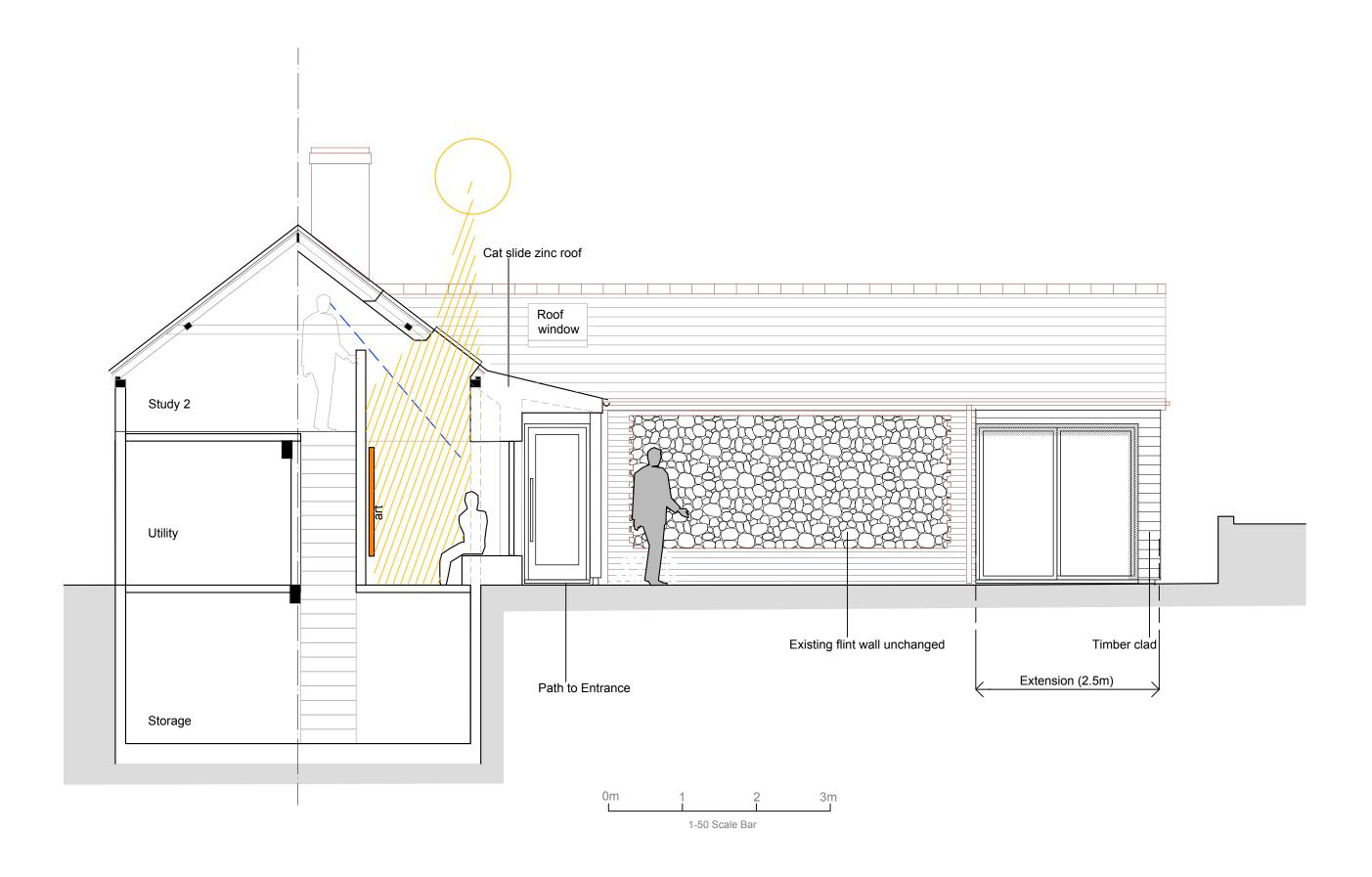
Proposed Schematic Section- West Elevation SCALE 1-50@A3
