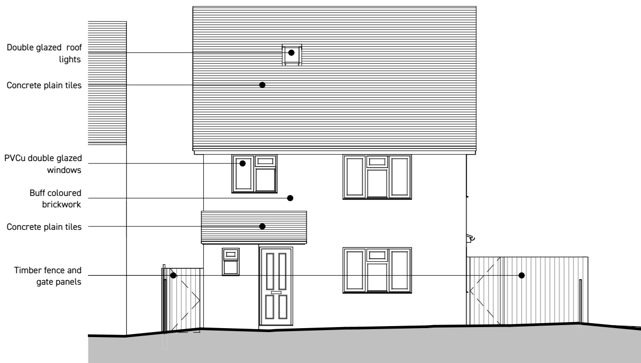
1 existing north elevation 1:100
