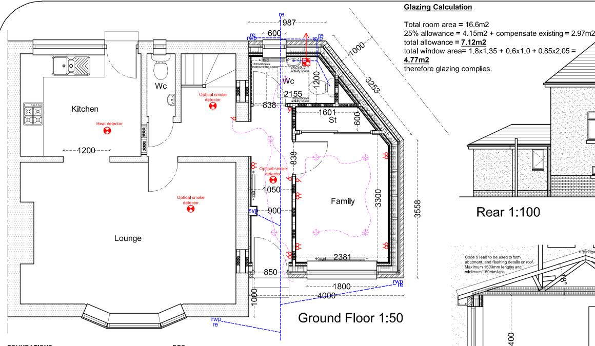
**FOUNDATIONS** Contractor to excavate and inspect existing foundations to ensure they are standard strip founds, if not structural engineer to be consulted prior to commencing main work. Contractor to excavate for founds and ensure they are down to a good bearing ground, and not to be formed on any made up ground. Any concerns regarding ground conditions to be
