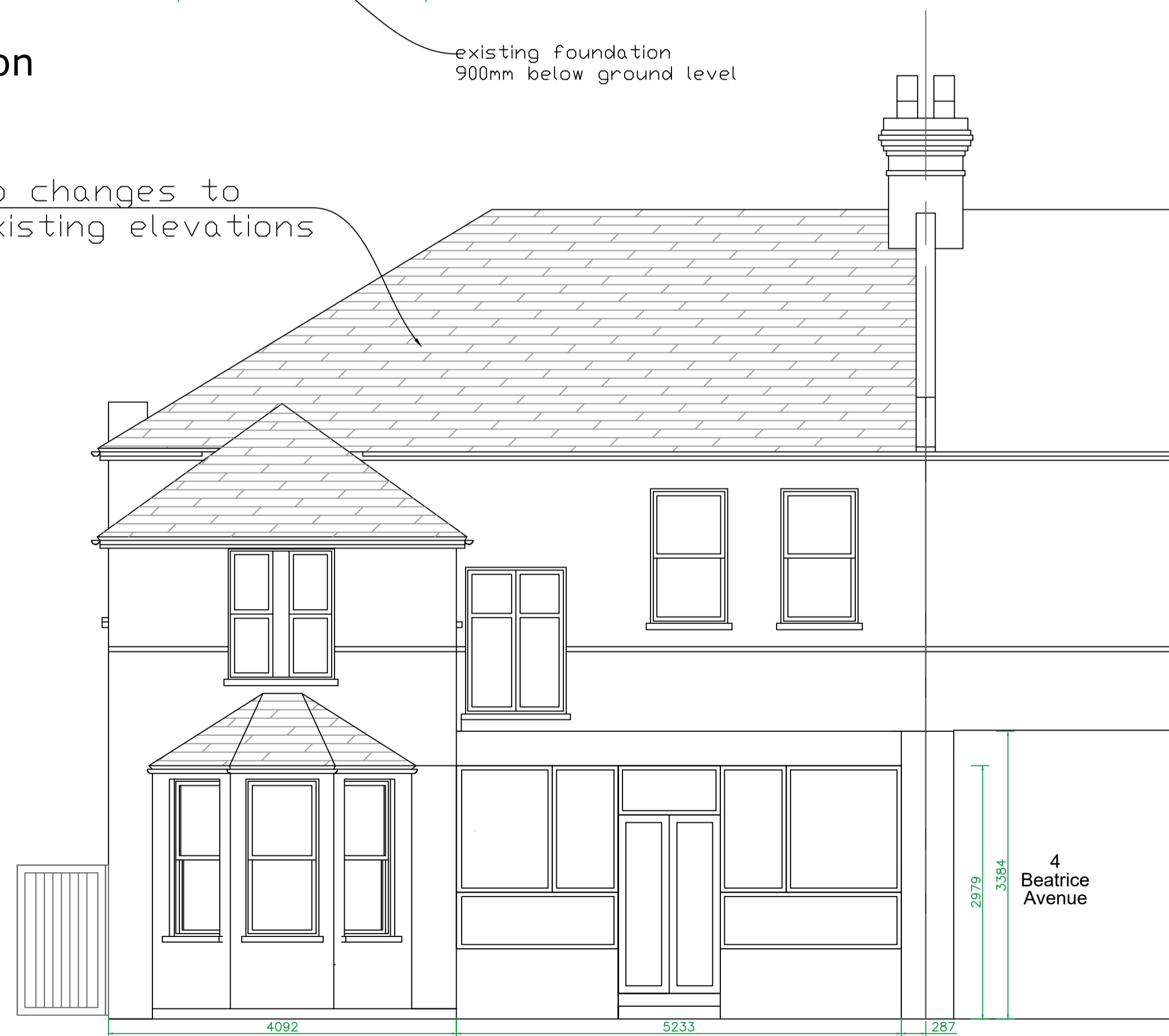
Existing Rear Elevation
