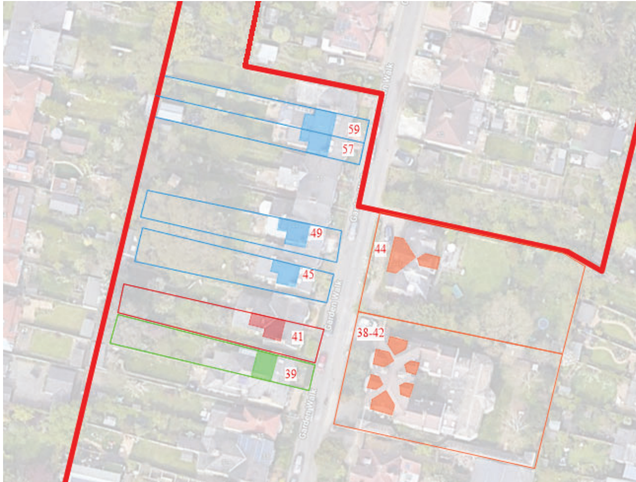
Fig 2.7: Map showing development at loft level to houses in immediate vicinity along Garden Walk. Blue= Properties which have extensions both over the main roof space and over the outrigger (up to rear chimney) via flat roofed dormers. Green= Property which has a box dormer to the rear, removing the original eaves and verge and with unscreened views onto no.41 rear garden. Orange= Properties which are a different style to no.41, with development at loft (2nd storey) facing N,E,S & W. Red= No.41 proposal Thick red line = boundary of Conservation Area
