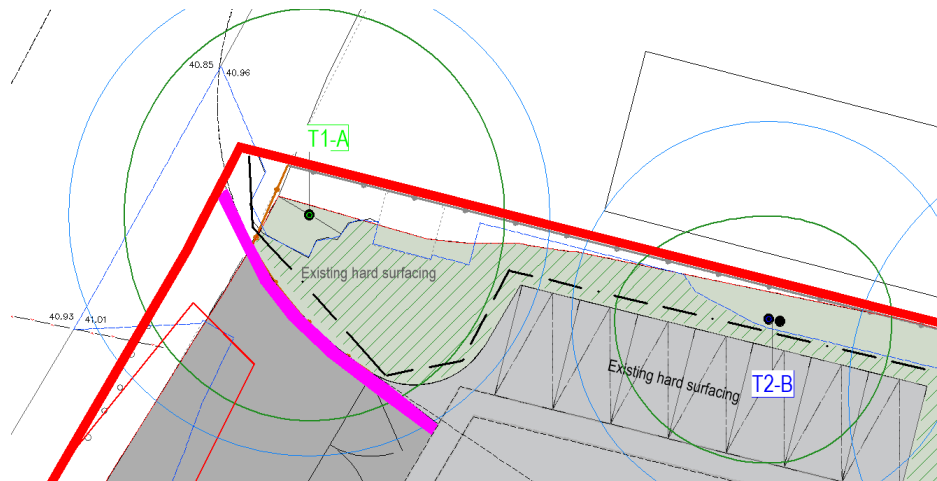
Plan 3 – extract from SHA 1730 TPPA. Do not scale, north is vertical. Pink is the kerb installation and green diagonal hatching is the area where Arboricultural Method Statement applies for lifting hard surfacing.
