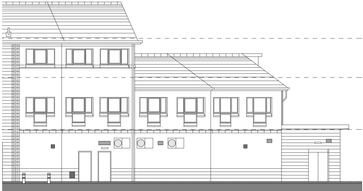
Drawing extract of existing elevation [North Elevation] demonstrating existing M&E and louvres on the facade.
