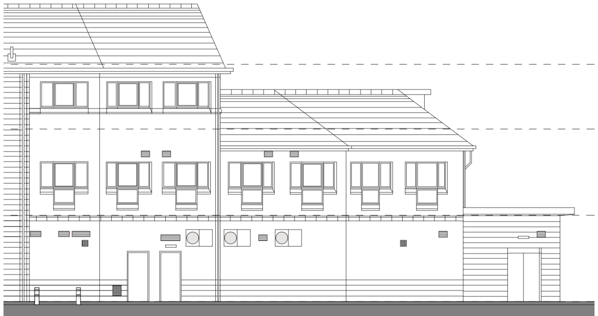
Drawing extract of proposed elevation [North Elevation] demonstrating new louvres blending with the existing M&E and louvres on the facade.
