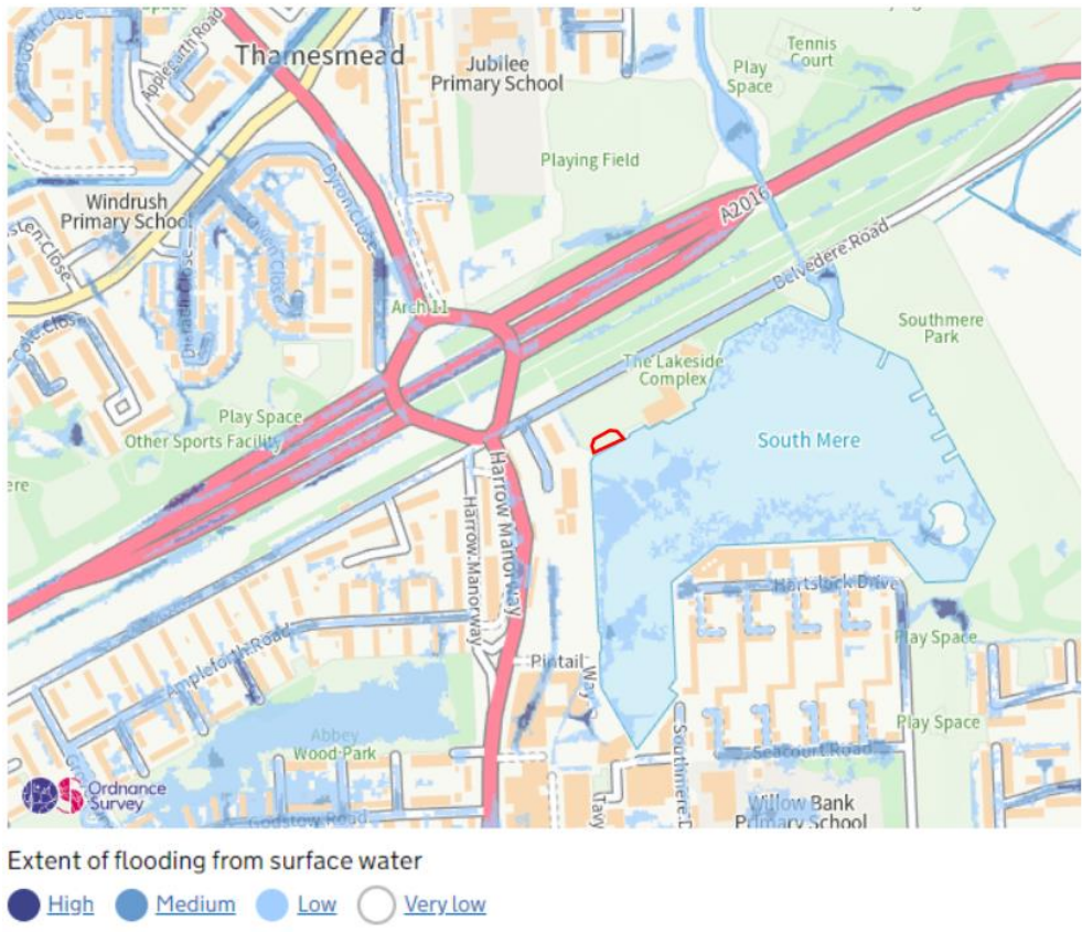
Figure 4.2: Environment Agency Surface Water Flood Risk Map
