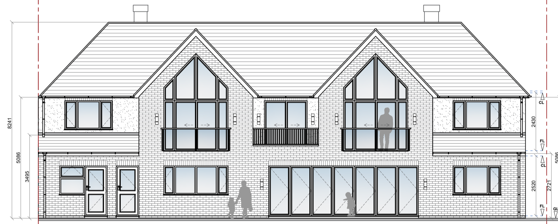
PROPOSED REAR ELEVATION SCALE: 1:100
