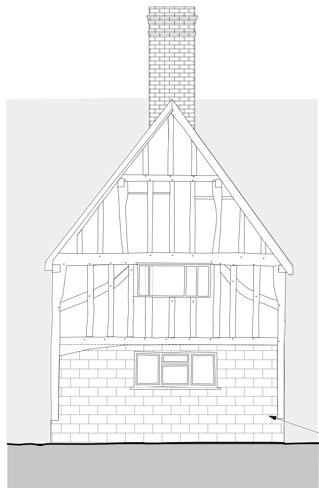
WEST ELEVATION / SECTION FRAME A-A
