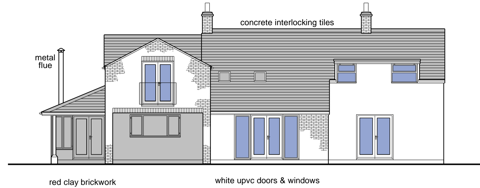
PROPOSED REAR/WEST ELEVATION 1:100
