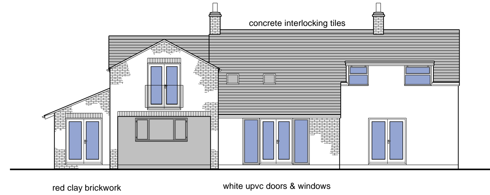
EXISTING REAR/WEST ELEVATION 1:100
