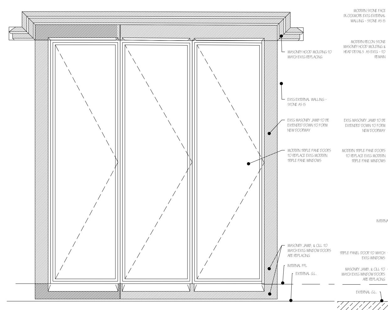
PROPOSED SECTION THRU. NEW DOORS - SCALE 1:100 @ A3
