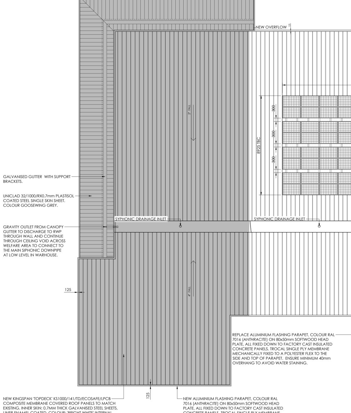
COMPOSITE MEMBRANE COVERED ROOF PANELS TO MATCH EXISTING. INNER SKIN: 0.7MM THICK GALVANISED STEEL SHEETS, LINER ENAMEL COATED, COLOUR: 'BRIGHT WHITE' INTERNAL FINISH. CORE: 141MM THICK ECOSAFE, LPC GRADE 'B', PIR INSULATION (UVALUE=0.21 W/M<sup>2</sup>K). OUTER CORE: 1.5MM THICK ARMOURPLAN PVC MEMBRANE, COLOUR: MID GREY (RAL 7046). ALL AS KINGSPAN LTD. PART 'L2' COMPLIANT RECOMMENDATIONS. EXTENT NOTED WITH GREY HATCH.
