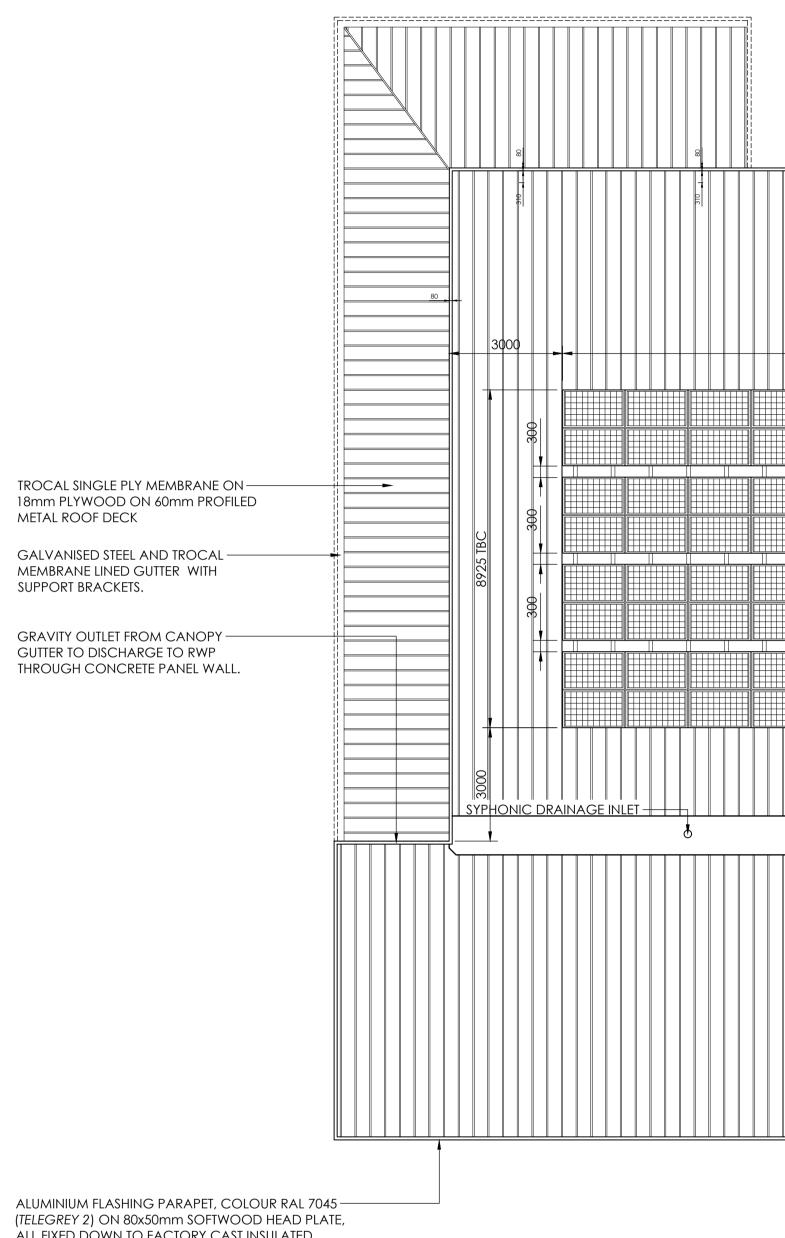
ALL FIXED DOWN TO FACTORY CAST INSULATED CONCRETE PANELS. TROCAL SINGLE PLY MEMBRANE MECHANICALLY FIXED TO A POLYESTER FLEX TO THE SIDE AND TOP OF PARAPET.
