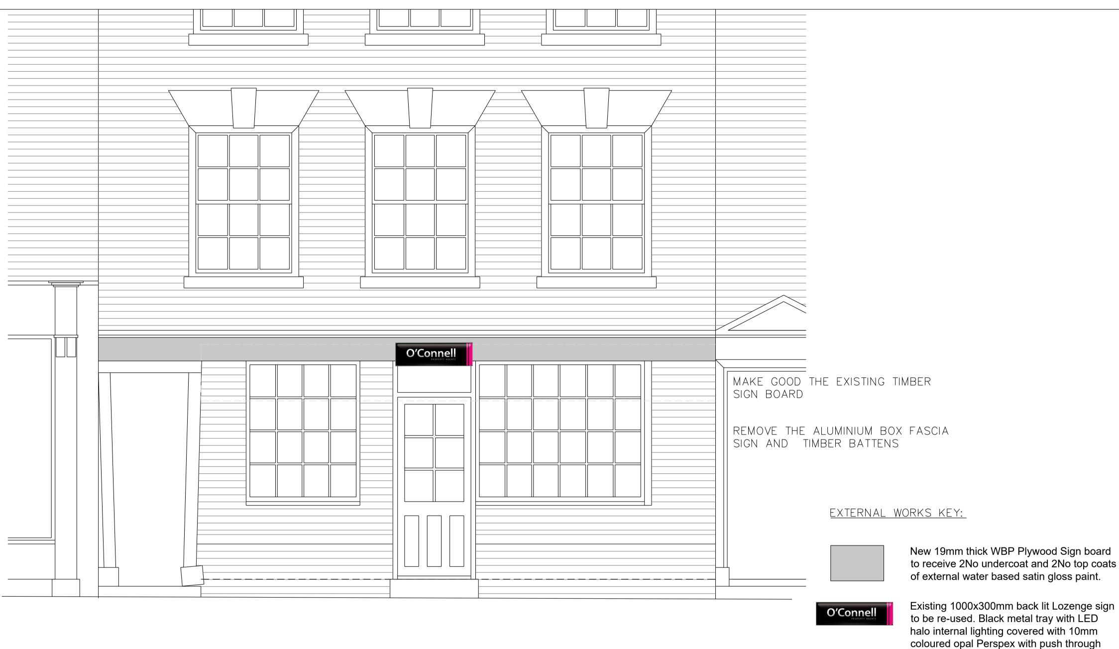
halo internal lighting covered with 10mm coloured opal Perspex with push through vinyl letters to give glow effect.
