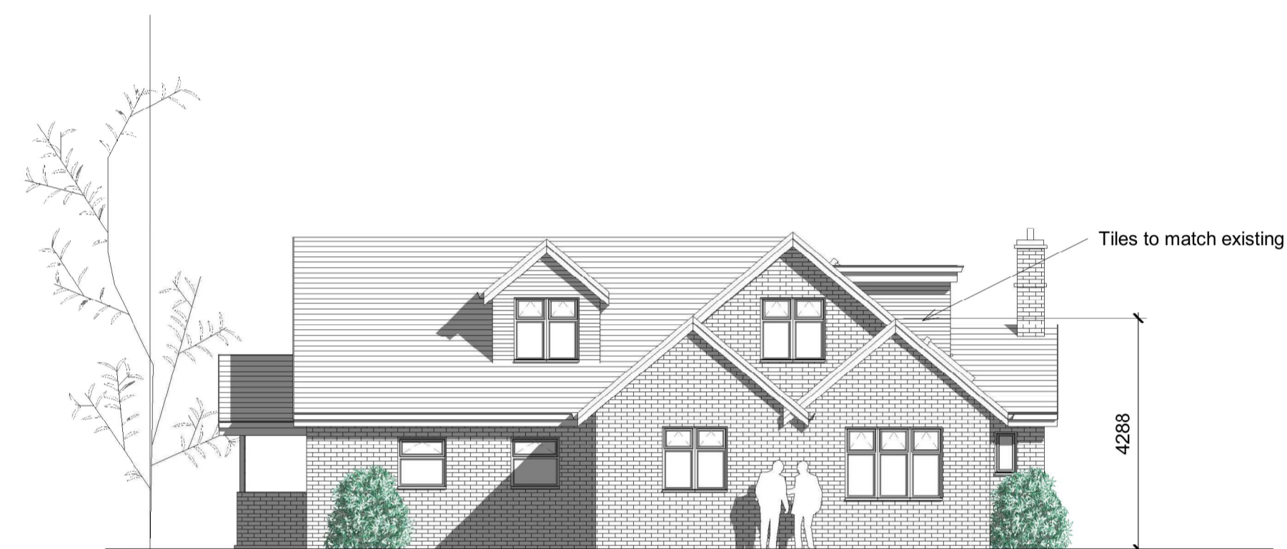
3 Side Elevation (North East) 1 : 100
