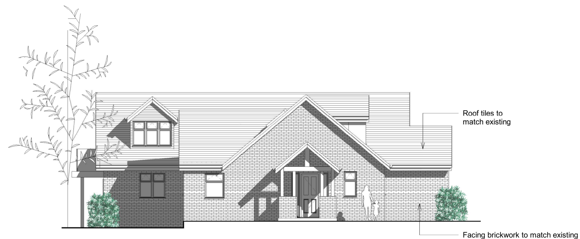
1 Front Elevation (South East) 1 : 100
