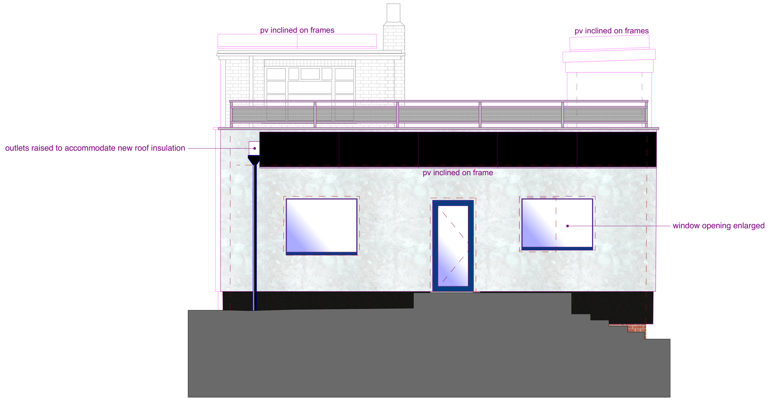
PROPOSED SIDE (South) Elevation 1:50
