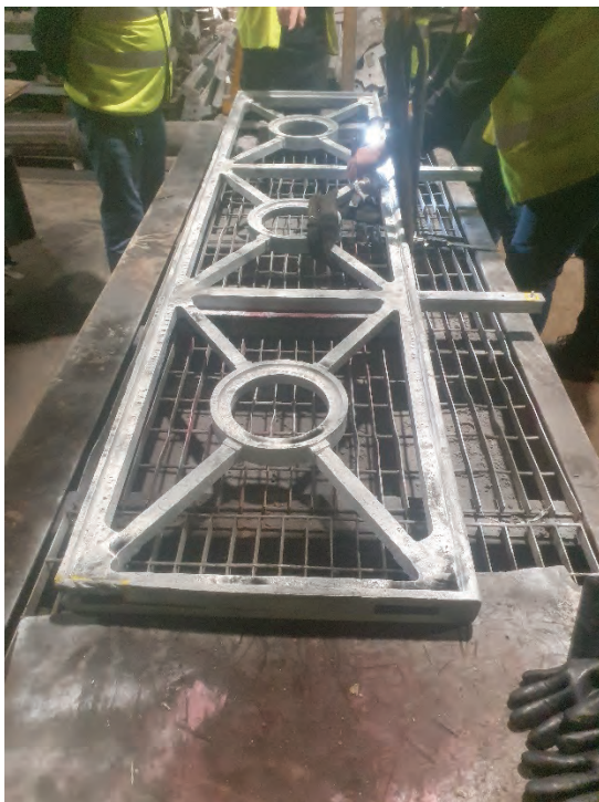
Photograph 12, infill panel after grit blasting during MPI inspection.
