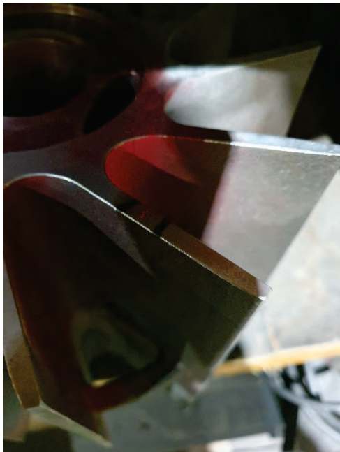
Photograph 3, indicating an example of a casting defect in a new casting that was to be remedied by fusion welding to achieve full specification.
