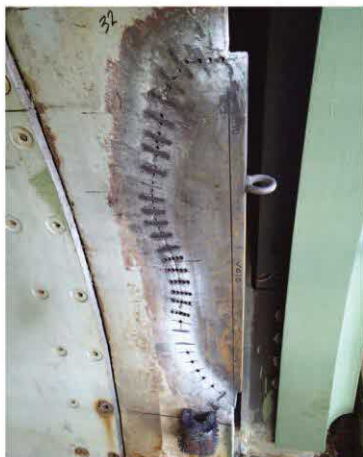
Figure 3 Example of cold stitching
