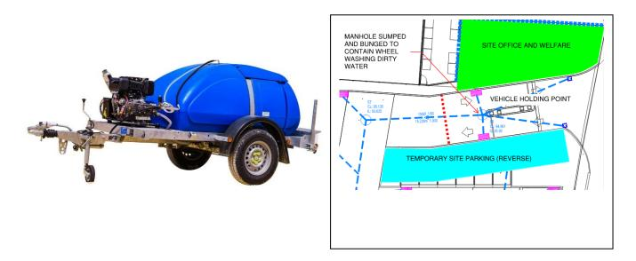
Proposed manhole S5 will be utilised bunged and sumped to contain dirty water run off and potential silting. Gullies to the site entrance will also act as water and silt catchment to prevent any run – off to Kingsway.
