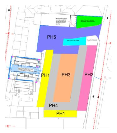
Materials for the permeable hard landscaping would be distributed via telehandler onto loading area for distribution around the working area.
