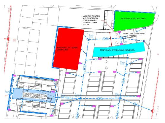
Excavated materials from attenuation excavation would be removed from site via wagons following access/egress routes amended during phased operation system via Kingsway Road. Vehicles to be directed on and off site by banksman.
