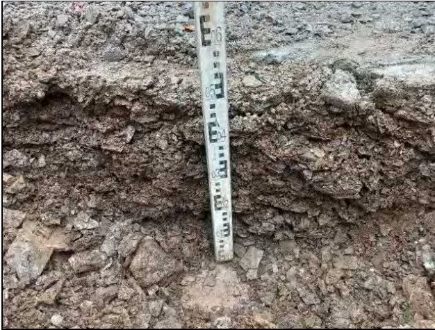
Plate 11: View showing 500mm capping thickness in TP0.
