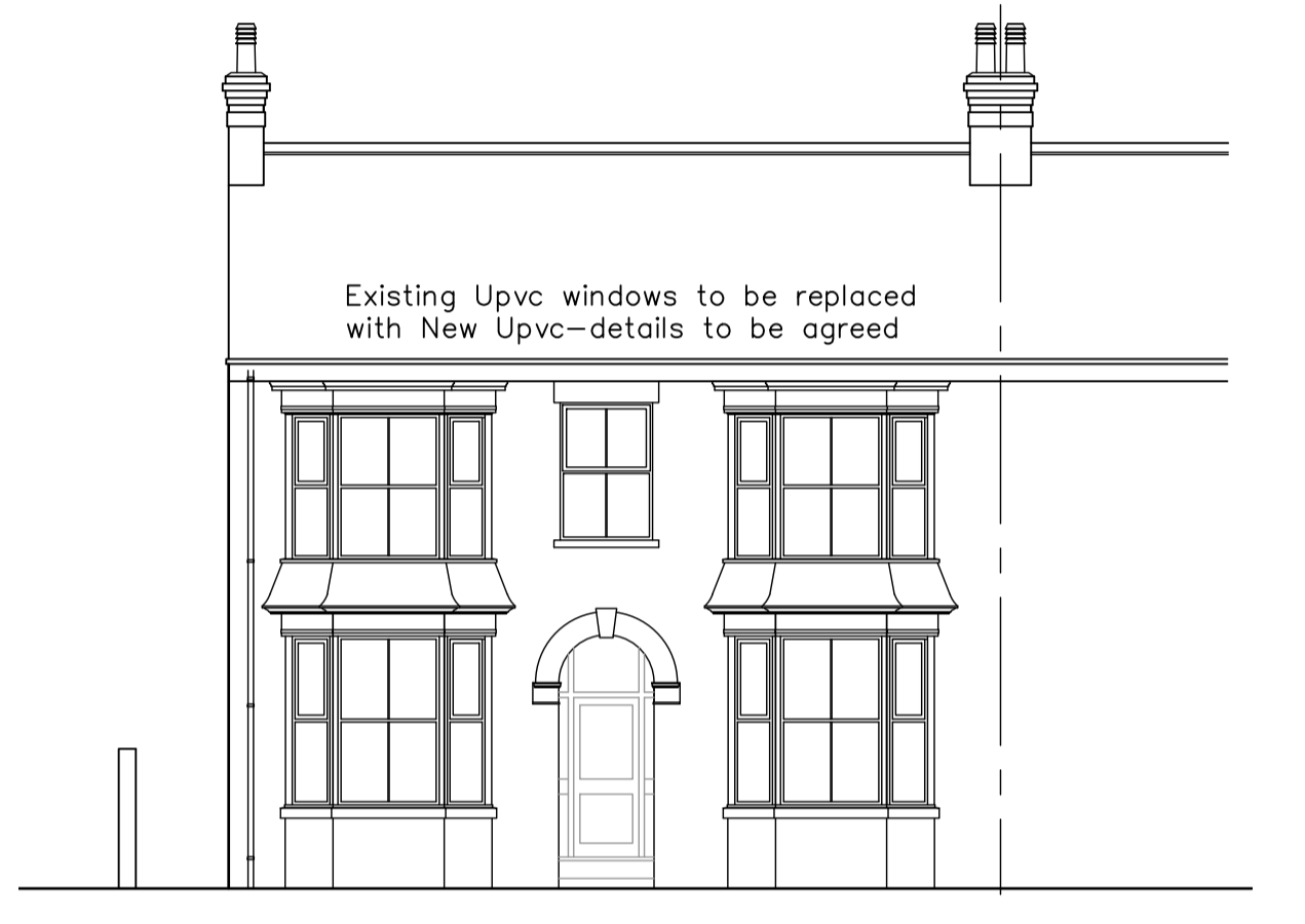
Existing Front Elevation
