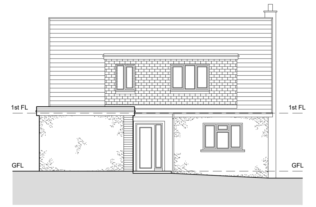
Existing Rear Elevation 1:100
