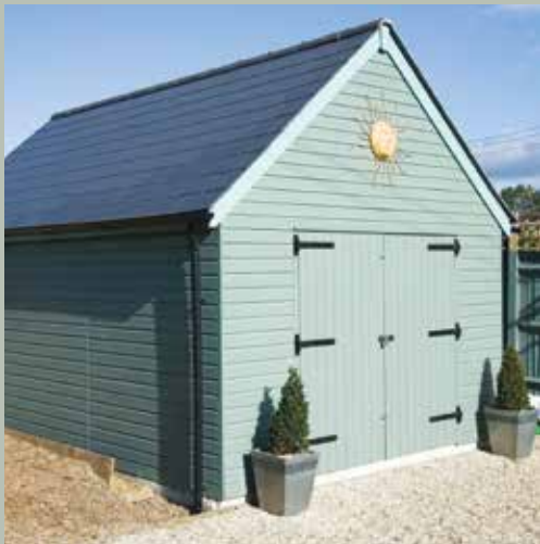
Single Garage. 35° fibre cement slate roof.
