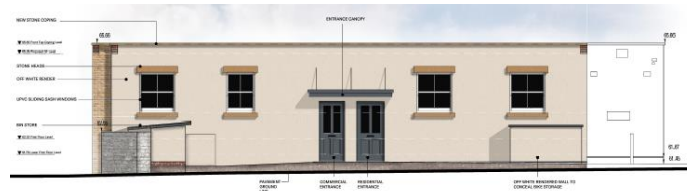
Approved rear elevation to a similar scale, note the rear of the building is just over one storey due to the height difference in ground levels to the front of the building
