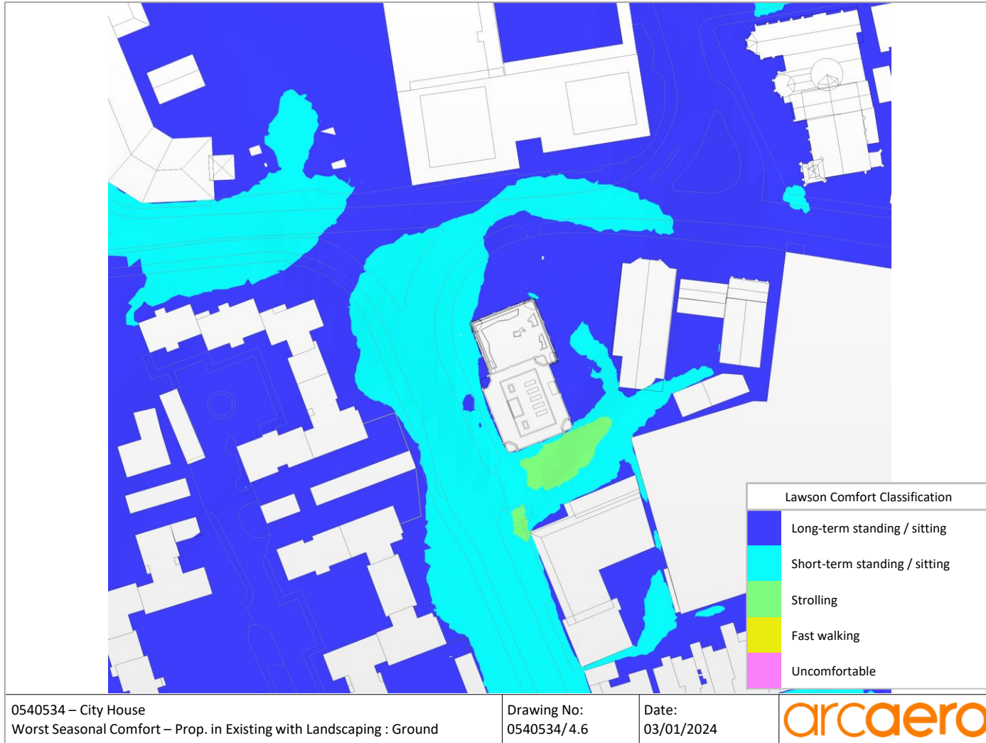
Figure 4.6 – Pedestrian wind conditions, proposed development within existing surrounds with soft landscaping, worst case season – ground level
