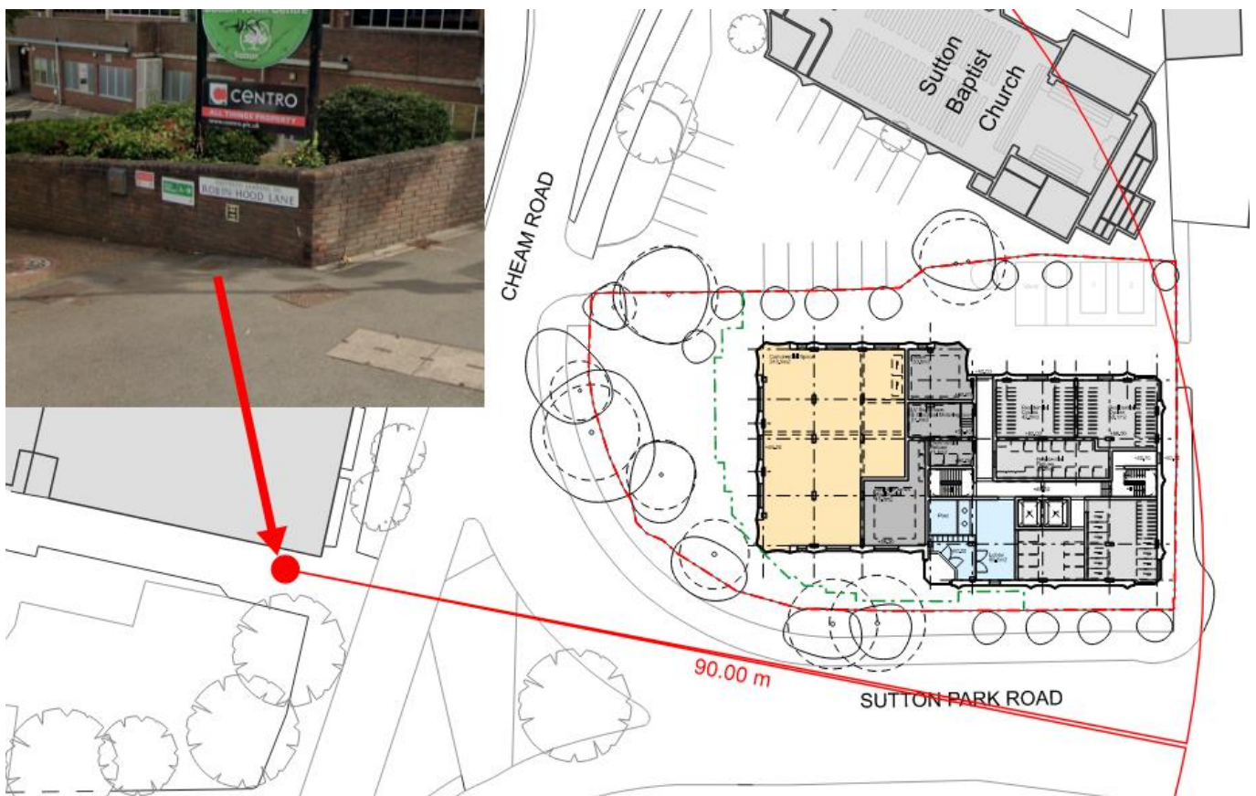
Figure 7-1111: Existing hydrant location in site vicinity
