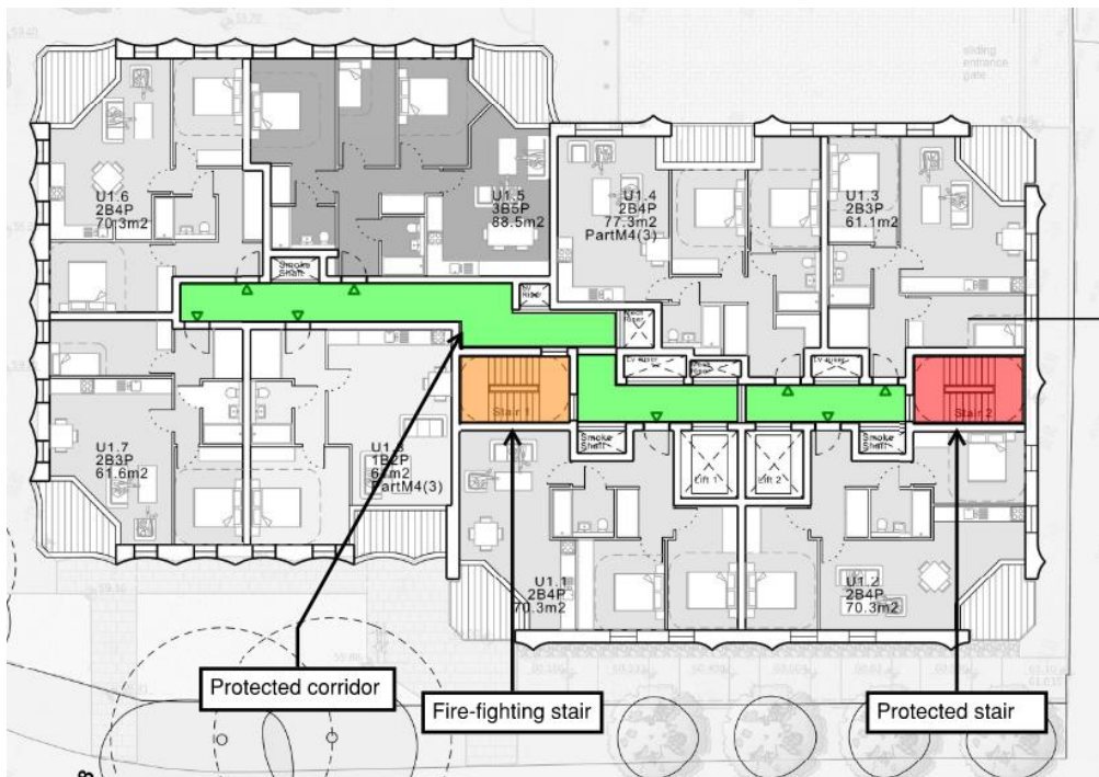
Figure 3-4444: Upper Floor Protected Escape Routes
