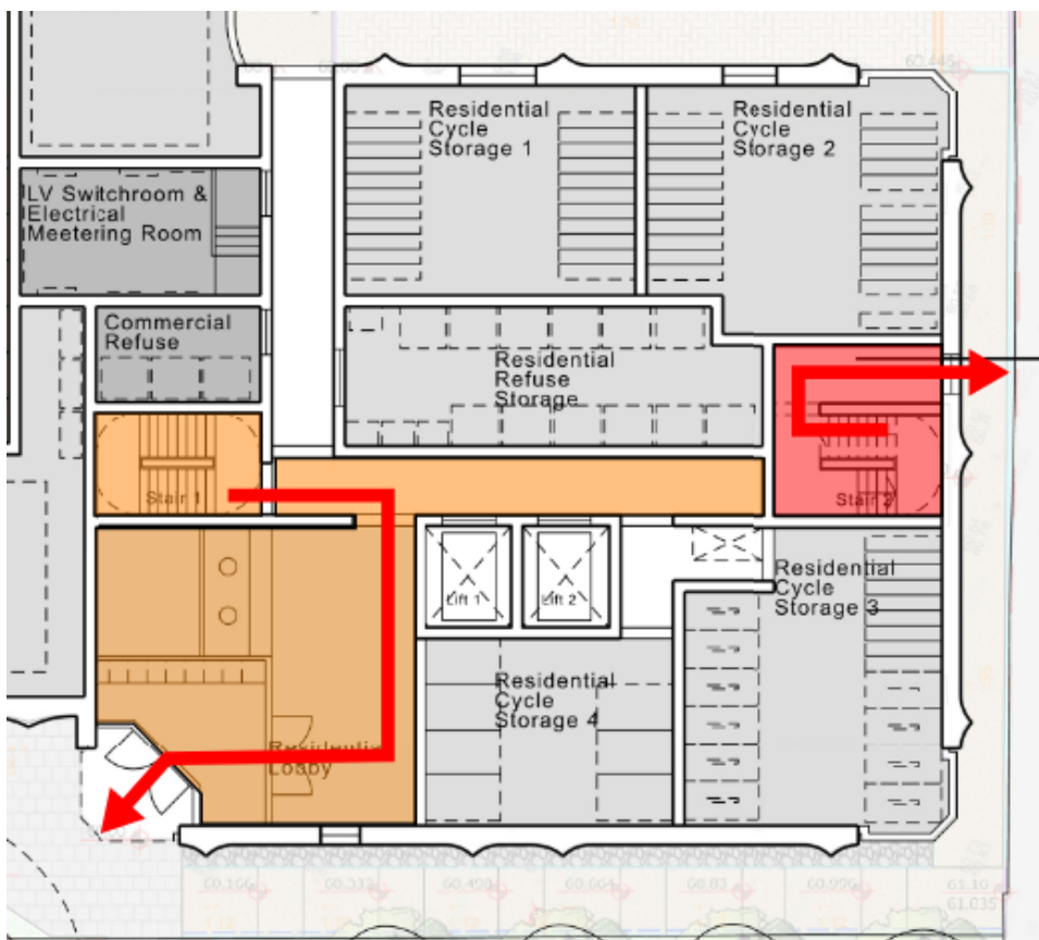
Figure 4-2222: Ground floor final exit routes
