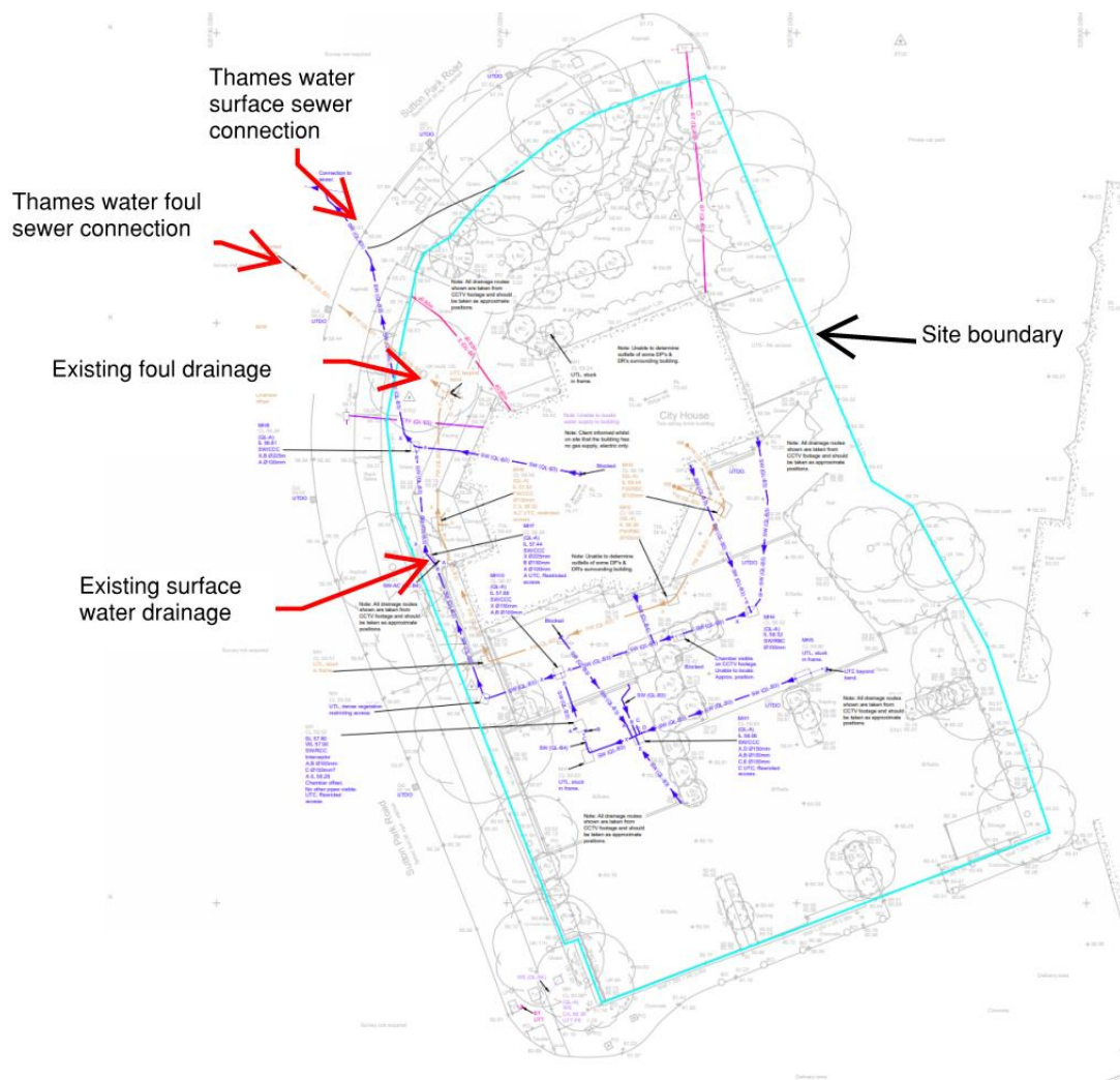
Figure 5: Existing drainage (Survey Solutions)
