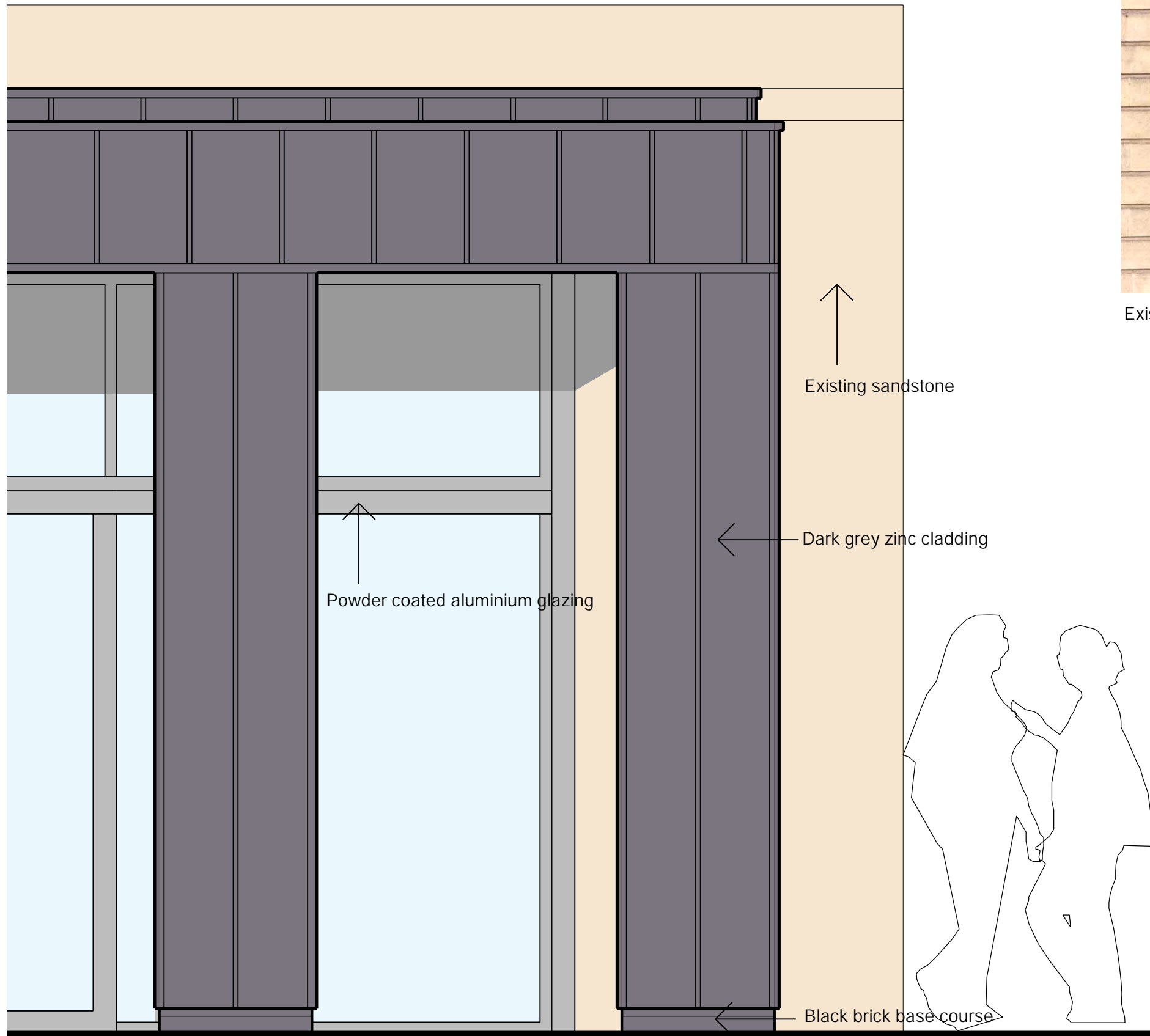
Canopy cladding detail 1:20
