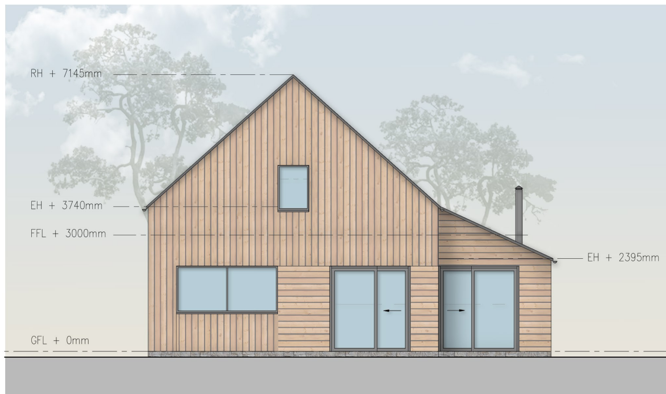
PROPOSED NORTH ELEVATION
