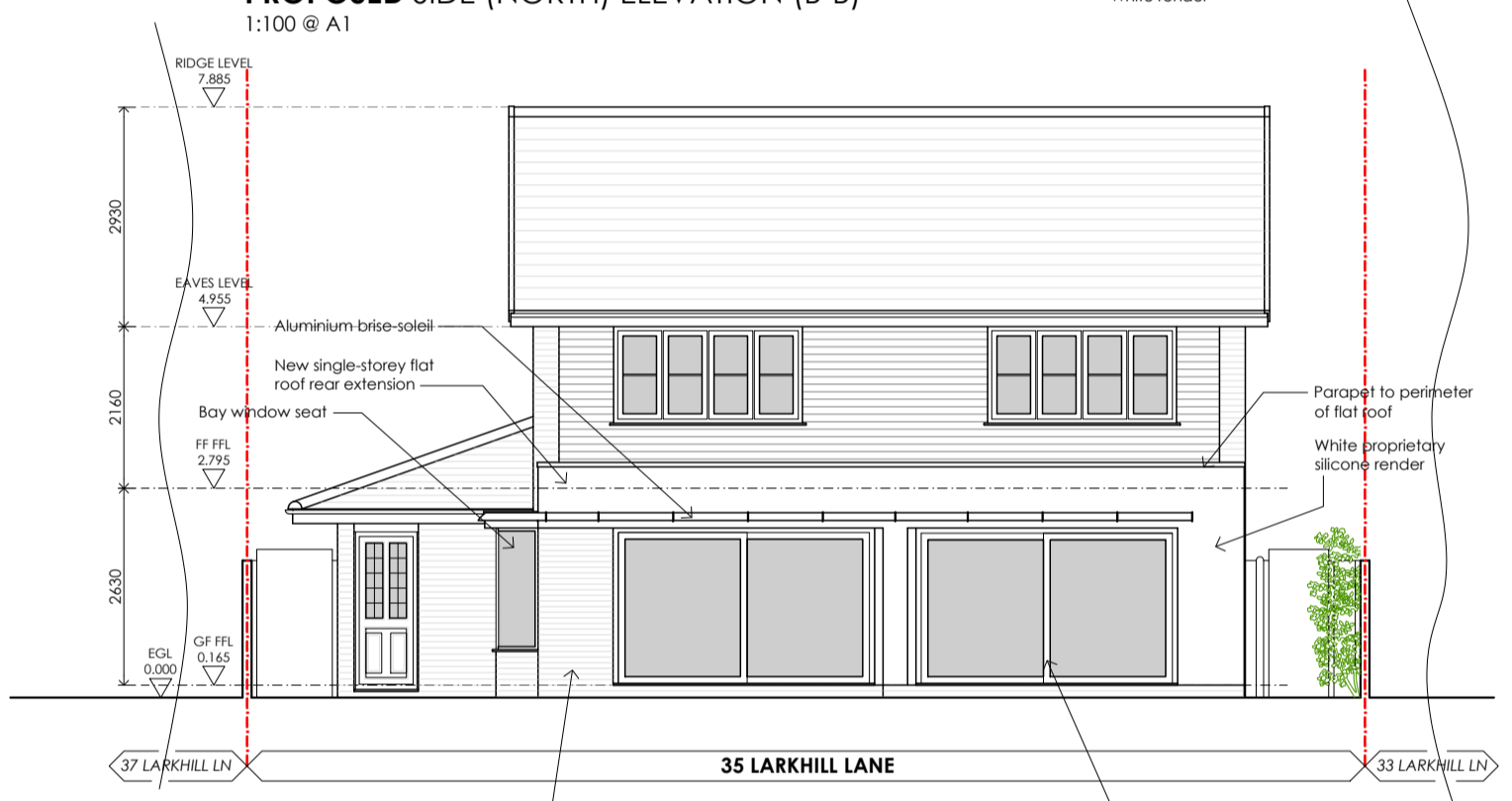
PROPOSED REAR (EAST) ELEVATION (C-C) 1:100 @ A1
