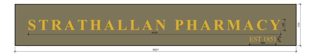
new non-illuminated fascia sign with olive green background (RAL 6013) and gold text detail, 5mm deep individual letters on 10mm locators to space off panel
