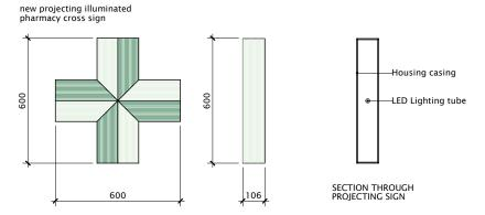
PROPOSED PROJECTING SIGN ELEVATIONS Scale 1:20
