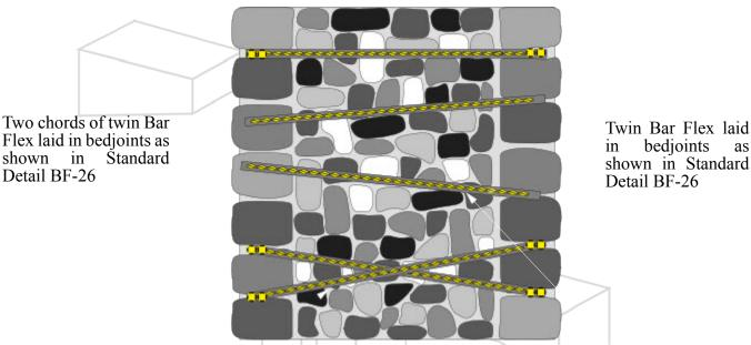
Cem Flex used to tie the opposite sides of the wall together and to act as a curtain walling system to stop the fill material above falling out.
