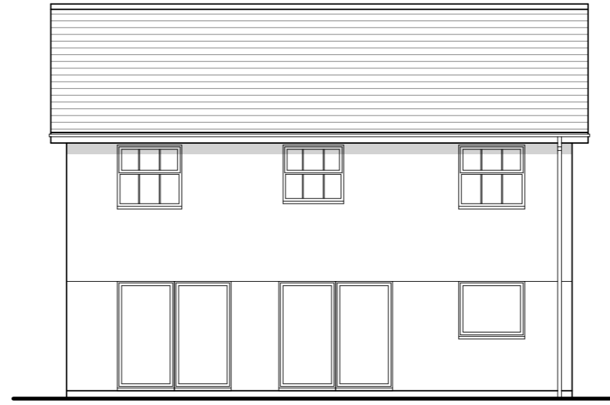
REAR ELEVATION AS EXISTING | Scale 1:100
