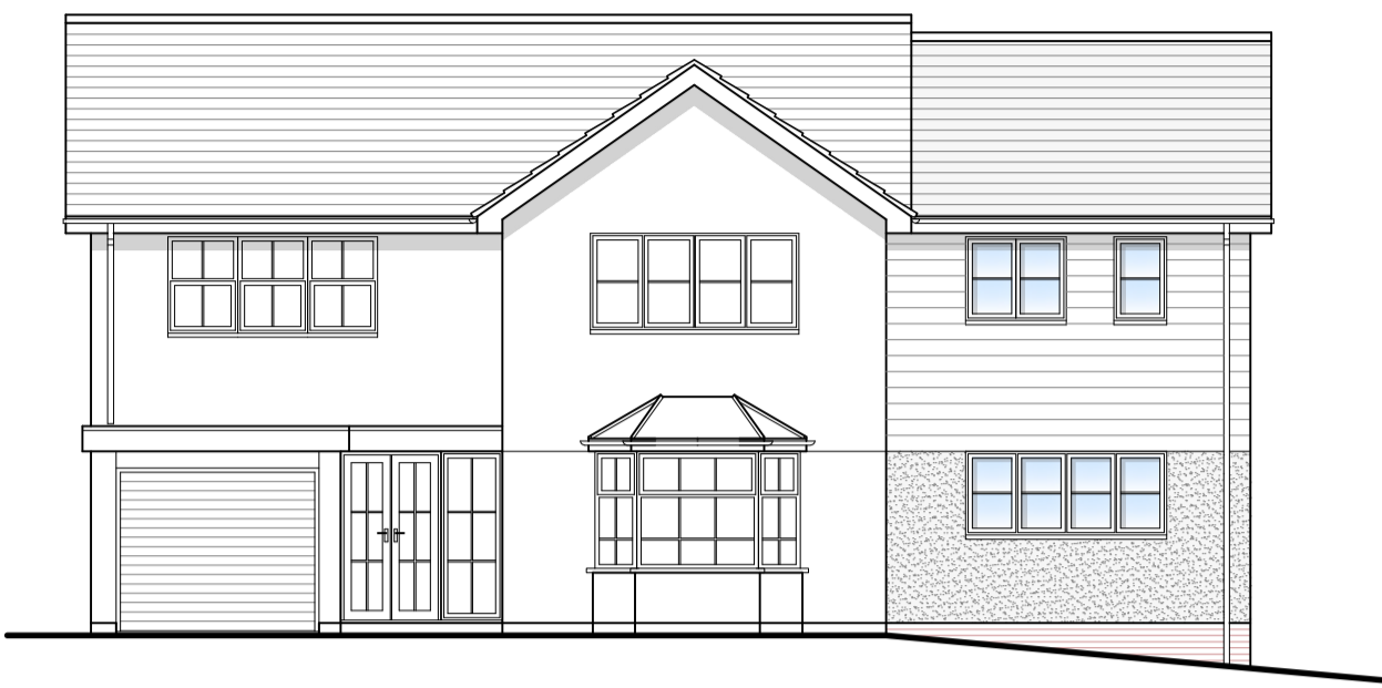
FRONT ELEVATION AS PROPOSED | Scale 1:100 Proposed extension to be rendered and clad in composite cladding colour: Anthracite Grey or similar
