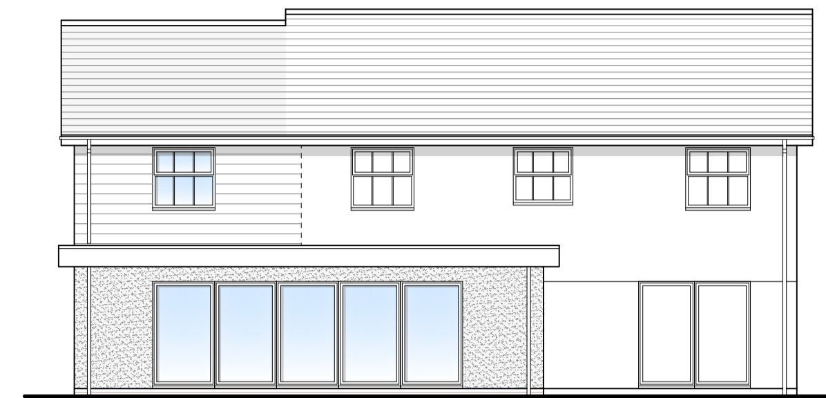
REAR ELEVATION AS PROPOSED | Scale 1:100
