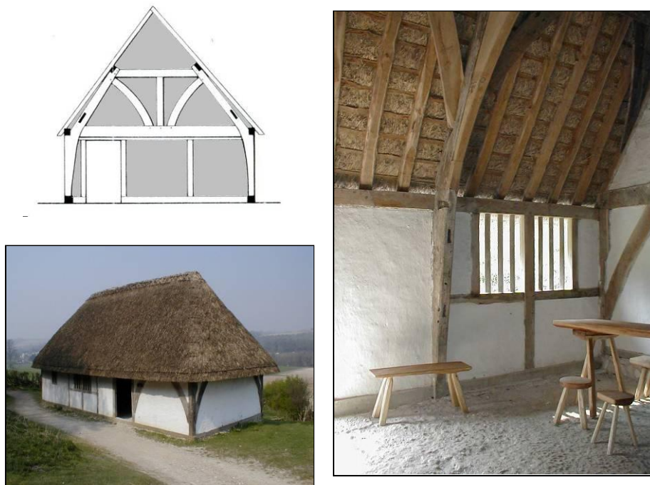
A section through a cruck building, with wattle-and-daub panels infill panels coloured grey (top left) and the house from Boarhunt (above left and right).
