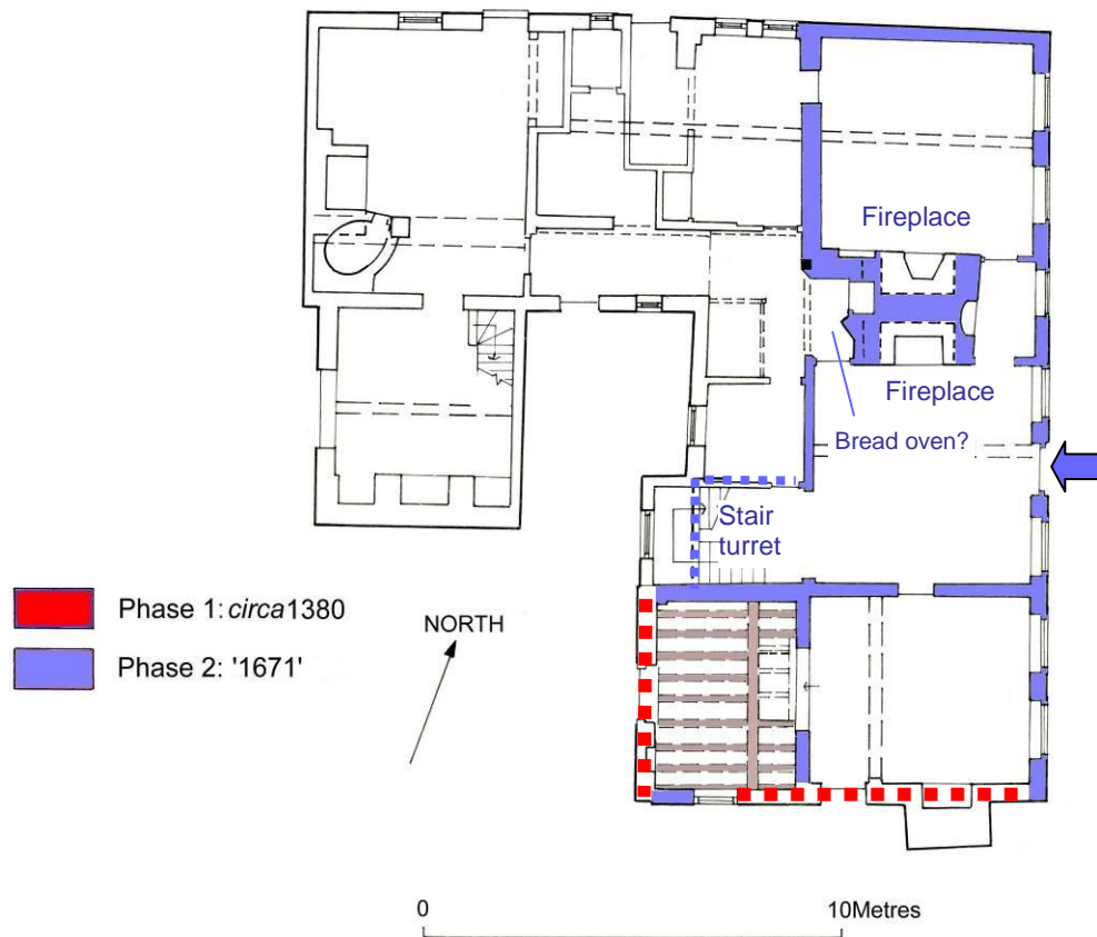
Ground floor plan, showing the arrangement of the extended (Phase 2) dwelling (dark blue). Scale 1:200.
