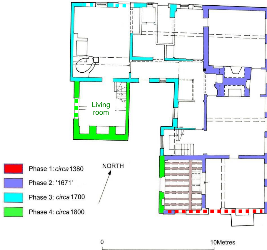
Ground floor plan, showing the arrangement of the extended (Phase 4) dwelling (green). Scale 1:200.
