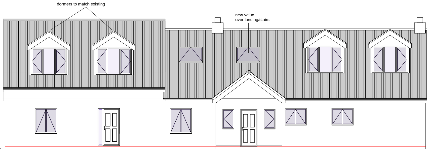
front elevation - north
