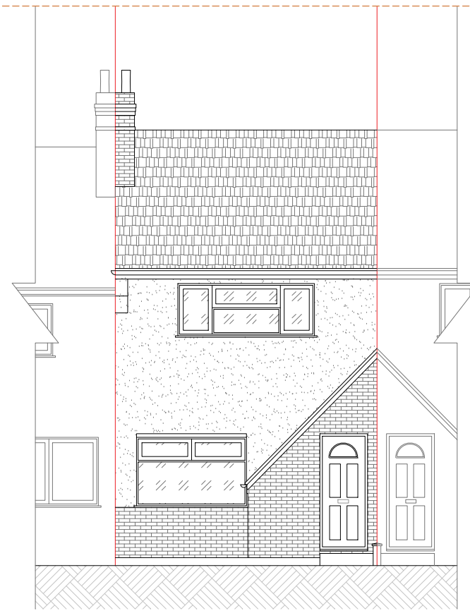
PROPOSED FRONT ELEVATION scale 1:100
